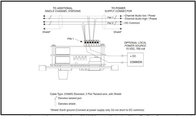
**FIGURE 8.** Audiocom mode connections for an SS-1002 Intercom Station in a U box. For Clear-Com connection, use the *Unbalanced Mode Intercom Channel* pin out information listed in "Specifications" on page 18.
